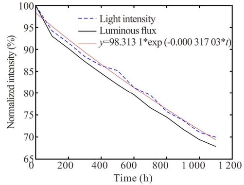
**Fig.3 Decay of light intensity and luminous flux of LED after aging at 200 °C**
