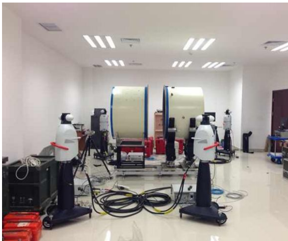
Fig.4 Experimental verification system for automatic docking of large sections
