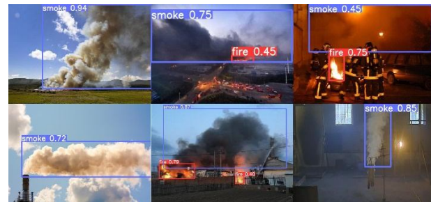
Fig.8 GAL-YOLOv5 detection results of suspected flame and smoke targets accompanied by environmental interference
