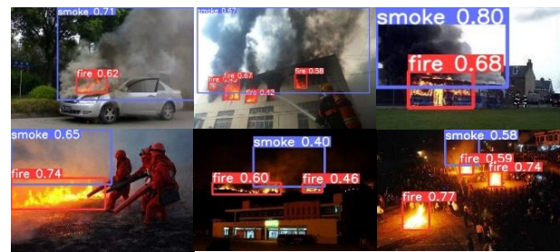
Fig.7 GAL-YOLOv5 detection results for prominent flame and smoke targets
