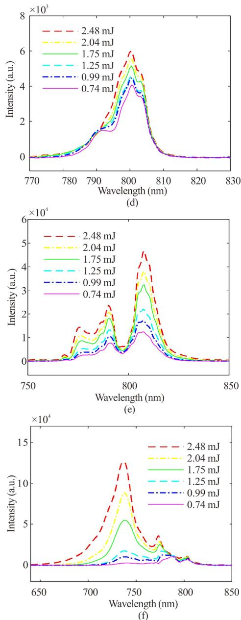
**Fig.2 Transmitted spectra of the focused femtosecond pulses with different initial energies at (a, c, e) 0.1 Pa and (b, d, f) 100 kPa when (a, b) BF<sub>1</sub> (790—820 nm) + NF (740—865 nm), (c, d) BF<sub>2</sub> (795—805 nm) + NF and (e, f) NF are used**
