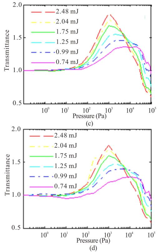
**Fig.5 Energy transmittance of the 800 nm femtosecond pulses with air pressure when (a, b) BF<sub>1</sub> and (c, d) BF<sub>2</sub> are used ((a, c) and (b, d) are measured by the spectrographic and photoelectric methods, respectively)**
