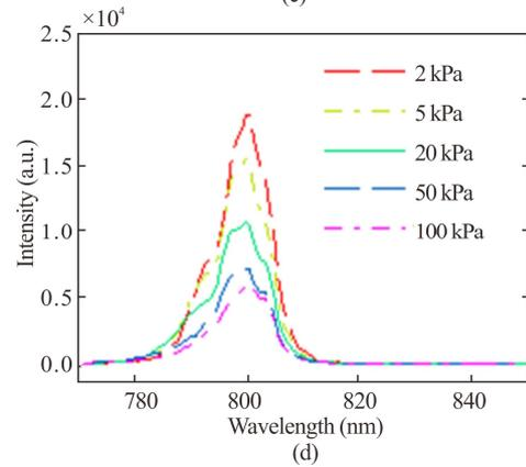
**Fig.3** Transmitted spectra of the focused femtosecond pulses whose energy is (a, c, e) 2.48 mJ and (b, d, f) 0.74 mJ at different air pressures measured when (a, b) BF<sub>1</sub> + NF, (c, d) BF<sub>2</sub> + NF, and (e, f) NF are used
