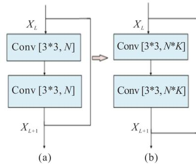
**Fig.2 Residual blocks: (a) Regular residual block; (b) Widened residual block**
