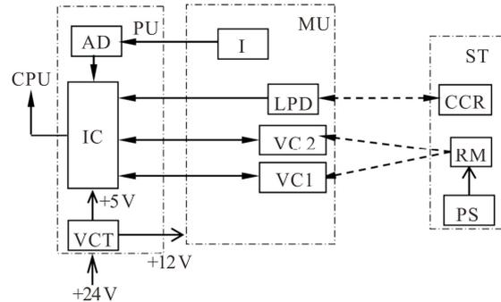
**Fig.3 Structure of the optic-electronics stereoscopic measuring system**
