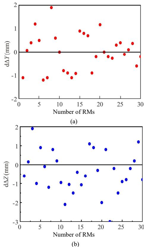
**Fig.9 Measuring errors of the tested system in real scene: (a) Y position of RM; (b) Z position of RM**
