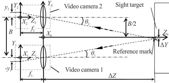
**Fig.2 Measuring scheme of the optics-electronic stereo system**
