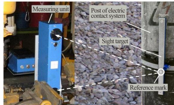
**Fig.8 Actual test picture of the optical-electronics stereo measuring system**
