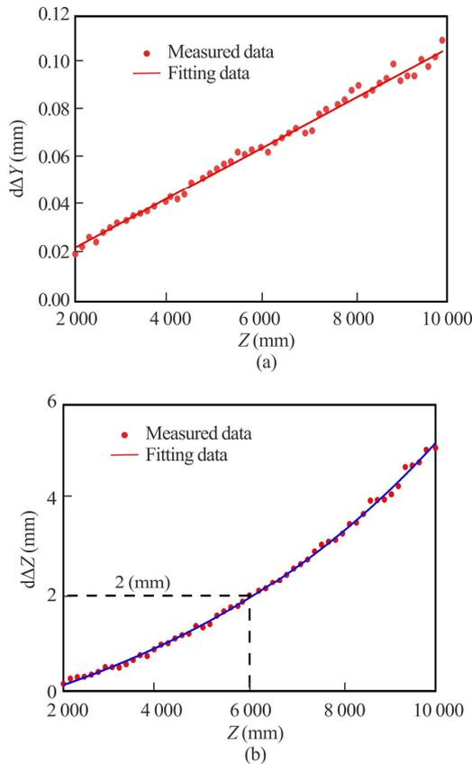
**Fig.7 Dynamic test results of the stereo system: (a) Vertical displacement measurement along the  $OY$  axis; (b) Horizontal displacement measurement along the  $OZ$  axis**
