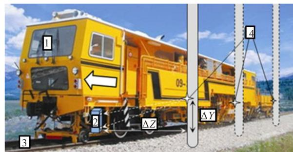
1: levelling-tamping machine; 2: MU; 3: track; 4: RMs
