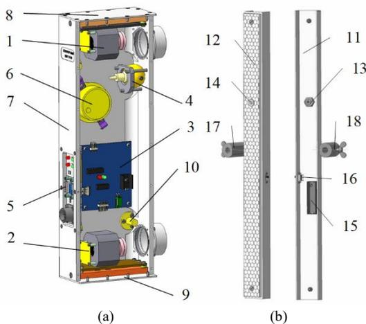
**Fig.4 Construction of (a) MU and (b) ST**
