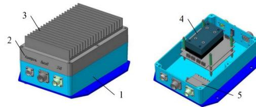
1: shell; 2: cover plate; 3: heat sink; 4: IC; 5: VCT
