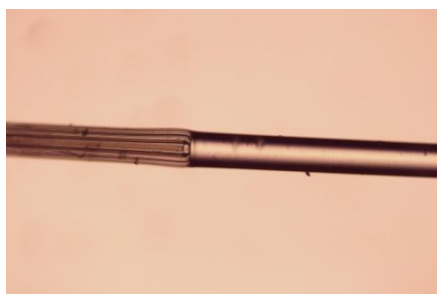
Fig.6 Fiber splicing end face
