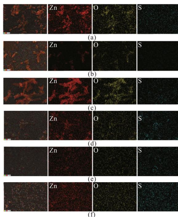
**Fig.3 EDS spectra of  $ZnO_{1-x}S_x$  films deposited with different ammonia concentrations: (a) 0.2 M; (b) 0.3 M; (c) 0.4 M; (d) 0.5 M; (e) 0.6 M; (f) 0.7 M**
