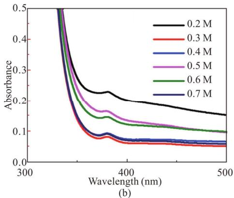
**Fig.5** Relationship between absorbance and wavelength of ZnO<sub>1-x</sub>S<sub>x</sub> films deposited with different ammonia concentrations in the wavelength ranges of (a) 300—900 nm and (b) 300—500 nm
