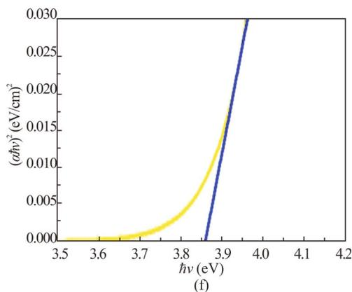
**Fig.7  $(\alpha\hbar\nu)^2$ - $\hbar\nu$  curves of corresponding samples under the ammonia concentrations of (a) 0.2 M, (b) 0.3 M, (c) 0.4 M, (d) 0.5 M, (e) 0.6 M, (f) 0.7 M**
