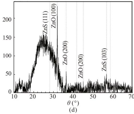
**Fig.4** (a) XRD patterns of the samples corresponding to 0.15—0.7 M ammonia water; XRD patterns of (b) Si (100), (c) Si (111), and (d) glass substrate deposition samples under the condition of 0.3 M ammonia, respectively
