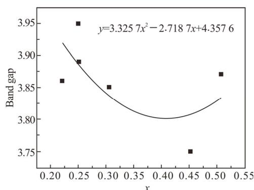
**Fig.8 Variation trend of band gap of  $\text{ZnO}_{1-x}\text{S}_x$  film with  $x$**
