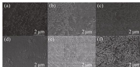
**Fig.2 SEM images of  $ZnO_{1-x}S_x$  films deposited with different ammonia concentrations: (a) 0.2 M; (b) 0.3 M; (c) 0.4 M; (d) 0.5 M; (e) 0.6 M; (f) 0.7 M**
