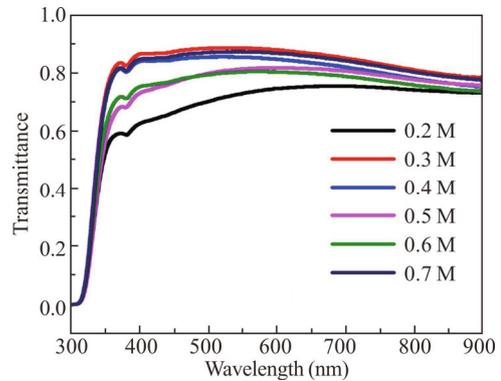
**Fig.6** Relationship between transmittance and wavelength of ZnO<sub>1-x</sub>S<sub>x</sub> films deposited with different ammonia concentrations
